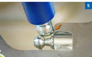
• Once the screws are tightened the leg brace should stay right above the ball and ball socket should touch the metal (see arrow).
