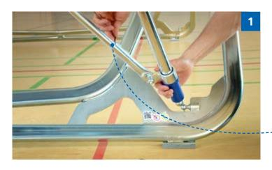
Loosen both allen screws on the small leg brace.
