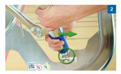
• Move the ball socket against the metal plate above the ball.
