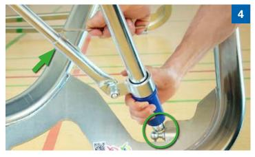
• Tighten both allen screws of the small leg brace while still pushing the leg brace up against the metal plate.
