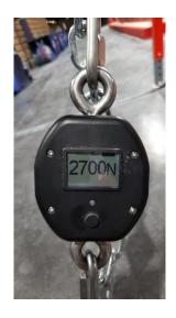
This easy to use tensiometer with measurement button and digital display **allows gymnasts to adapt the tension of the cables of the apparatus according to their needs** in competition as well as in training.
